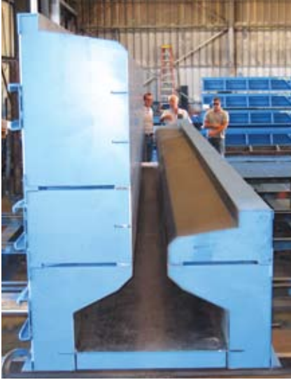
The new beam section can vary in depth from 70 in. on the left to 28 in. on the right.
