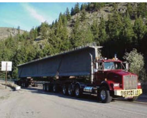
Transporting WSDOT's "Super Girder."
