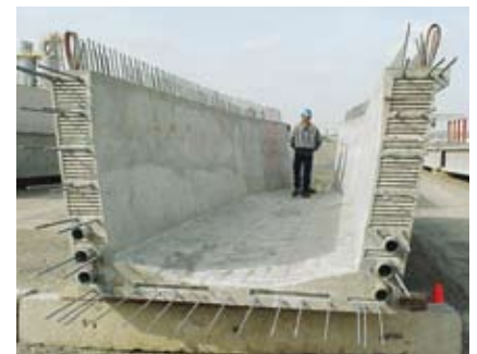
Precast trapezoidal tub girder.
