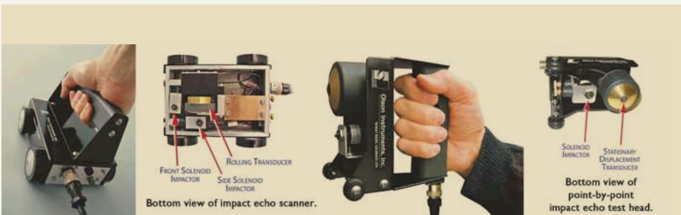
Handheld impact echo scanner device, traditional point-by-point impact echo unit.
