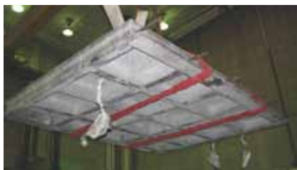
A laboratory test deck panel like the ones being used for Little Cedar Creek Bridge in Wapello County, Iowa. Photo: Iowa State University.
