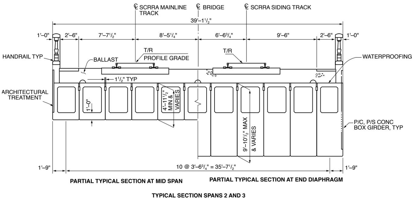
Typical section of the Haven Avenue Grade Separation Bridge in one of the main spans. Drawing: PBS&J, an Atkins company.
