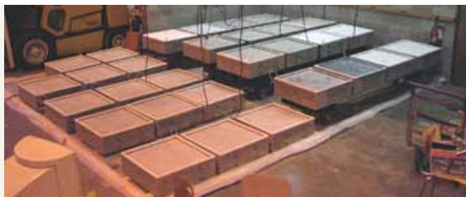
Thirty laboratory test specimens were subjected to 6 months of accelerated corrosion testing. Photo: University of Wisconsin-Milwaukee.
