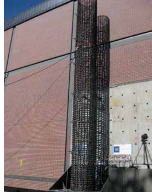
View of test Specimen II having a 34 ft height and 3 ft 8 in. diameter.
