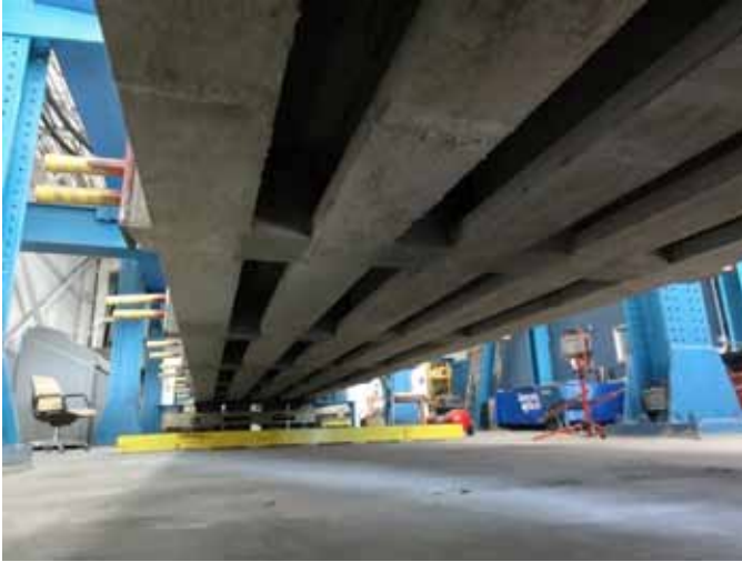
A scaled model of a deck bulb-tee bridge, 40 ft long and 14 in. deep, is shown in the structures laboratory of Lawrence Technological University and following testing to failure. The bridge uses carbon fiber prestressing strands, all nonmetallic reinforcement, and UHPC in the longitudinal joints. Photo: Lawrence Technological University.
