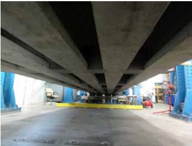
A scaled model of a deck bulb-tee bridge, 40 ft long and 14 in. deep, is shown in the structures laboratory of Lawrence Technological University and following testing to failure. The bridge uses carbon fiber prestressing strands, all nonmetallic reinforcement, and UHPC in the longitudinal joints. Photo: Lawrence Technological University.
