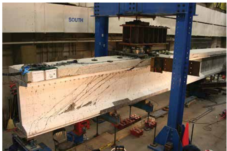
Shear test of lightweight concrete prestressed girder at Turner-Fairbank Highway Research Center. Photo: Gary Greene, PSI Inc.
