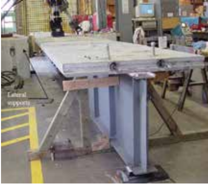
Wisconsin laboratory test beam for fatigue cycling. Photo: University of Wisconsin.
