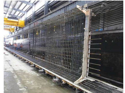
A 205-ft-long girder used for the Alaskan Way Viaduct using bundled harped strands. Photo: Concrete Technology Corporation.
