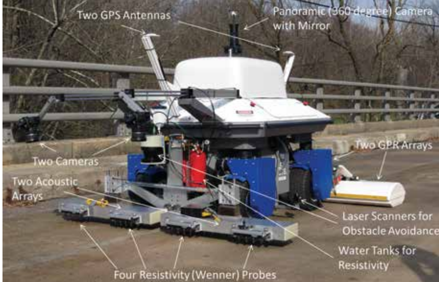
Robot components of the RABIT™ bridge deck assessment tool expedites field data collection. Photo: Rutgers University.
