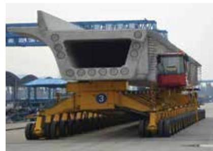
Tire trolley for 900-kip, single-track box girders. Photo: BWM.
