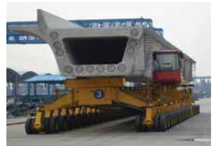
Tire trolley for 900-kip, single-track box girders. Photo: BWM.
