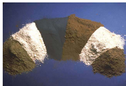
Supplemental cementitious materials enhance the performance properties of concrete. From left to right, Class C fly ash, metakaolin, silica fume, Class F fly ash, slag cement, and calcined shale. Photo: Portland Cement Association.
