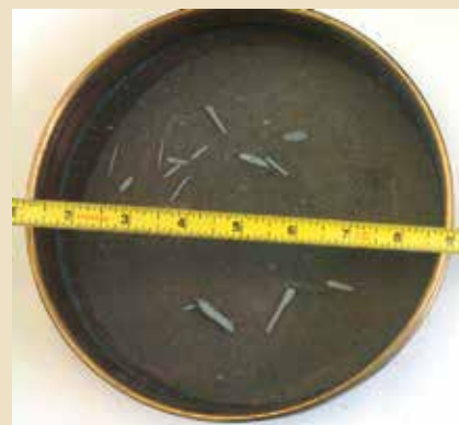
Debris from silica fume containing an average of approximately 1.5% of particles over 45µm.
