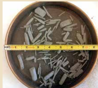
This photo shows typical +45µm particles found in raw silica fume. (Percent is unknown.) All photos: Elkem Materials Inc.
