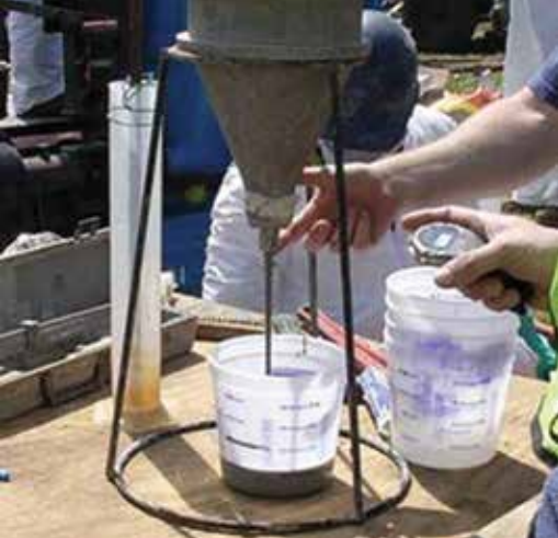
Figure 2. The wet density and flowability are tested at mixer as well as at the the outlet.
