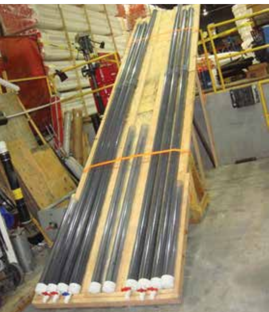
Figure 1. The inclined tube test is a large scale bleed test. All Photos: Structural / VSL.
