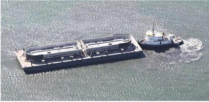
Barging of the precast concrete components that were used to construct the 3.1-mile-long Tappan Zee Bridge in New York. The precast concrete open-footing tubs were set on drilled shafts and filled with concrete to create the bases for the bridge's piers. Photo: Bayshore Concrete.
