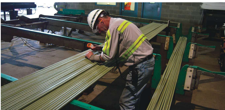
Measurement of coating thickness as part of the plant quality-control procedures. Photo: Epoxy Interest Group of CRSI.
