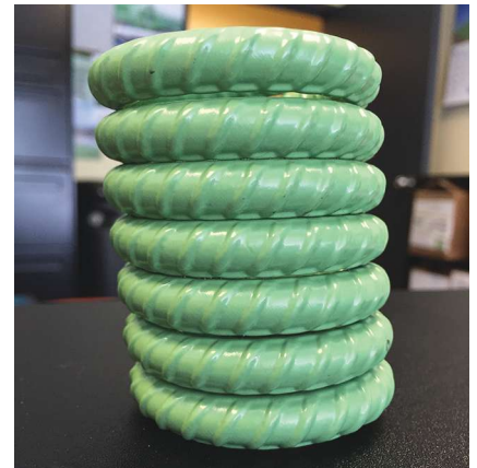
A typical example of epoxy coating flexibility. This No. 4 bar is bent around a 1.5-in.-diameter pin. No cracking of the coating is observed. Photo: David McDonald.
