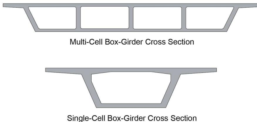
Figure 1. Typical concrete box-girder cross section. All Figures: Developed by Corven Engineering for the Federal Highway Administration.
