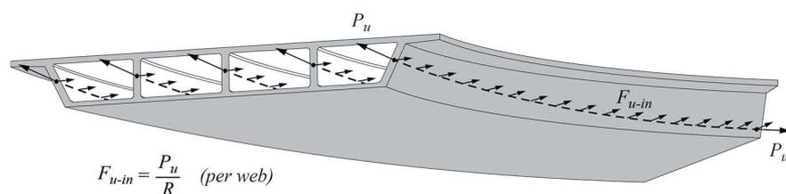
Figure 4. Effects of tendons in curved concrete members.
