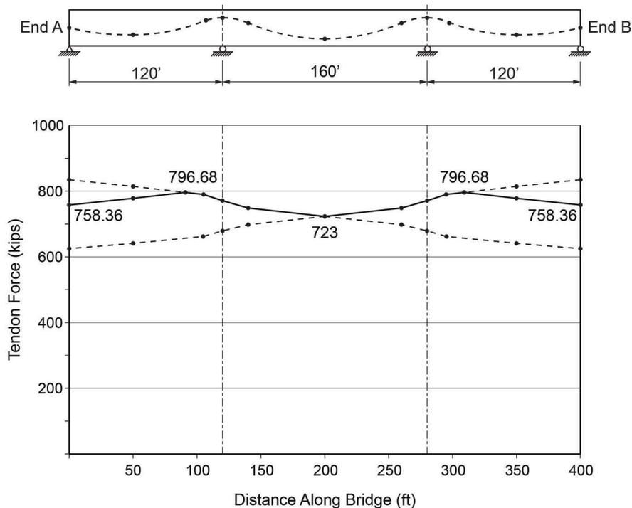
Figure 3. Tendon force diagram after stressing from both ends.
