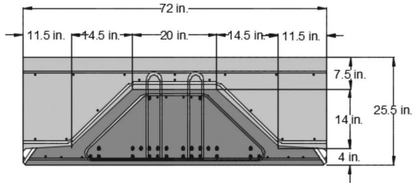
Typical composite cross section dimensions of a inverted-tee beam used for the US 360 Bridge, Figure: Virginia Department of Transportation.
