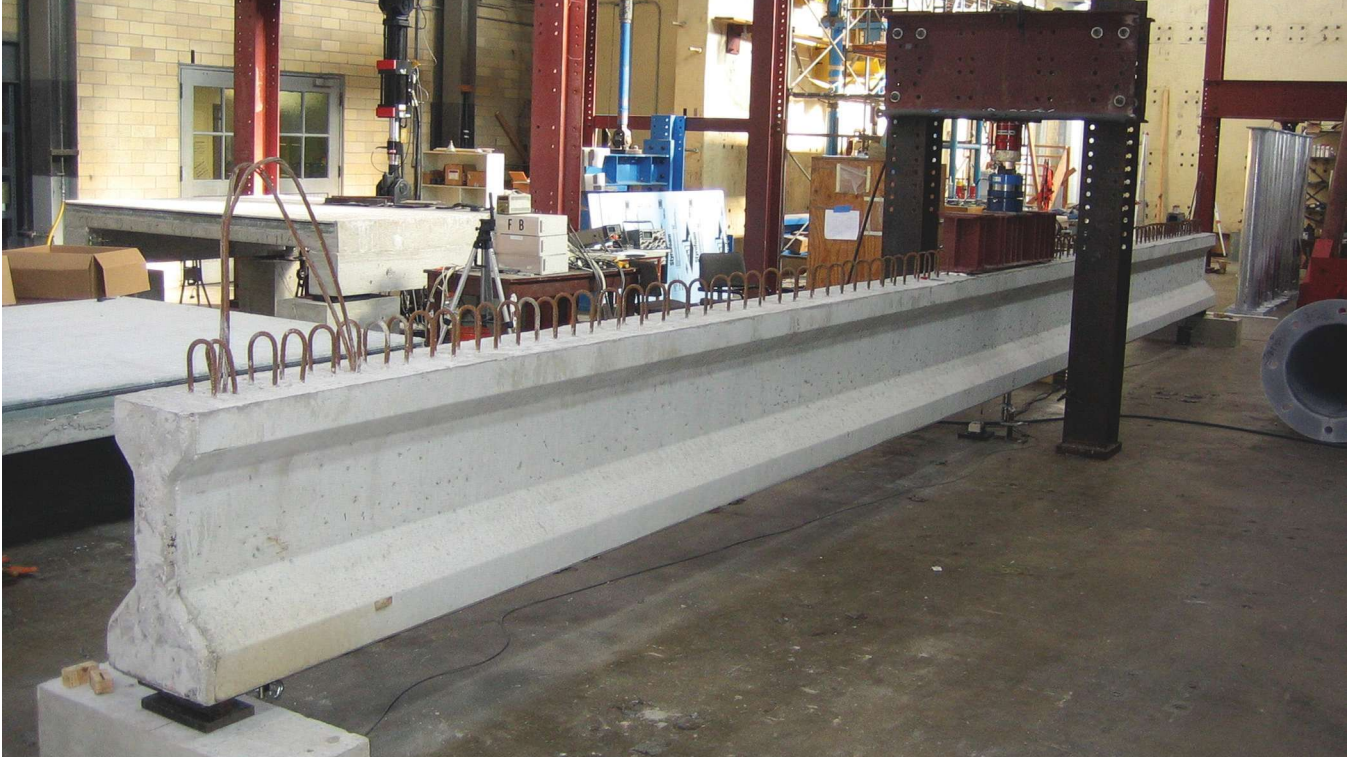
Service load testing of a beam in the lab. Photo: David B. Birrcher.
