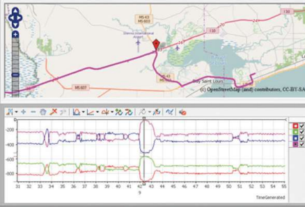
Data fusion of traditional strain plots, with synchronized time-lapse video, geolocation map, and interpolated three-dimensional sensor mapping.
