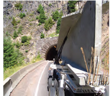
A heavy haul truck uses the Salt Creek Tunnel. The truck transports a girder through the east portal to another project. Photo: Knife River Corporation.
