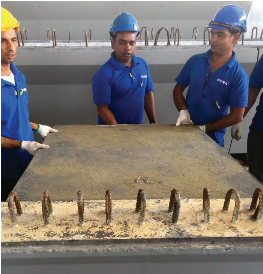
DURA Technology's stay-in-place precast concrete deck form panel. Photo: Precast/Prestressed Concrete Institute.
