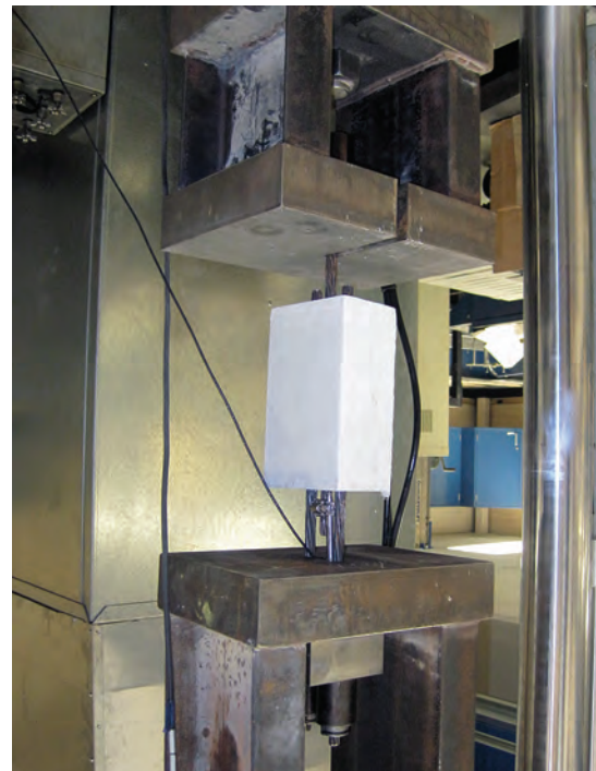
Lap-splice test of untensioned strands in ultra-high-performance concrete. Photo: Federal Highway Administration.
