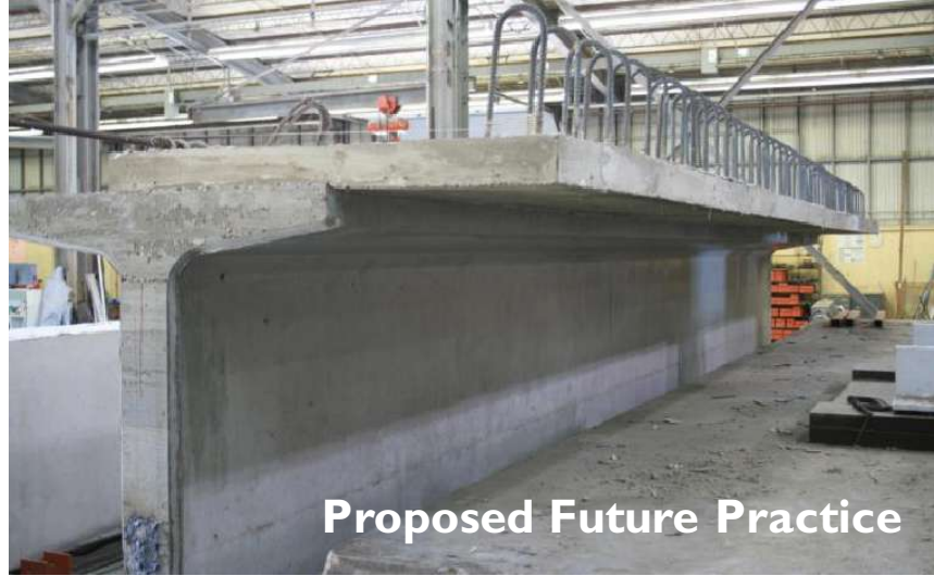
Figure 1. The current deck overhang bracket system and the proposed precast concrete overhang system.. All Figures and Photos: Sean P. Clifton.
