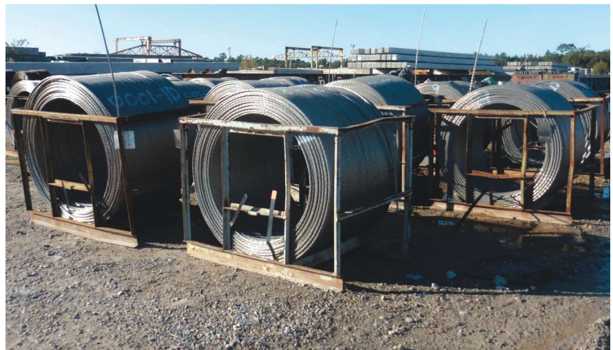
Packs of stainless steel strand to be used in the production of prestressed concrete piles.
