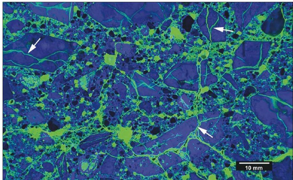
can combine this technique with image analysis to provide more robust, quantitative measurements of capillary porosity," he explains. "It allows us to measure on a pixel-by-pixel basis the capillary porosity of the concrete. That allows us to evaluate quantitatively how various aspects of the construction process, ranging from consolidation to finishing to curing, affect the microstructure of concrete."
