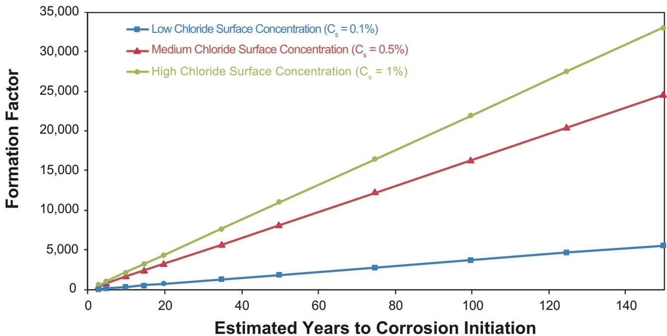
An example of the relationship between formation factor and predicted service life. Note: C<sub>s</sub> = the concentration of chlorides in solutions in contact with concrete. Figure developed from an approach described by Spragg.<sup>1,2</sup>
