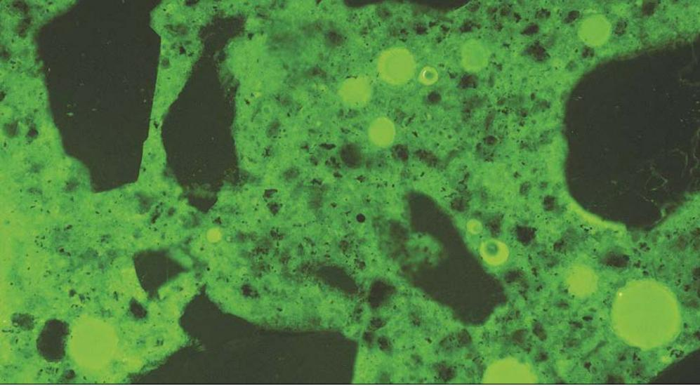
A transmitted fluorescent-light photomicrograph showing detail of the cement paste in a thin section. The bright-green circles are air voids that have 100% porosity, and the black areas are aggregate particles with essentially 0% porosity. The variations between these colors represent variations in the paste's capillary porosity.
