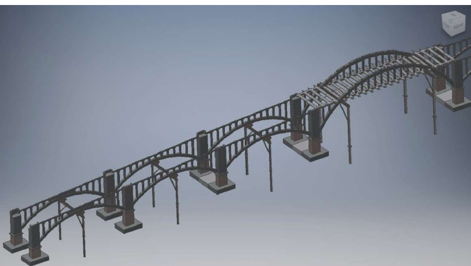
Integrated three-dimensional bridge model in software with temporary construction supports shown. Figure: FINLEY Engineering Group.
