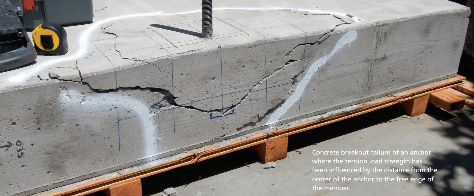
Concrete breakout failure of an anchor where the tension load strength has been influenced by the distance from the center of the anchor to the free edge of the member.
