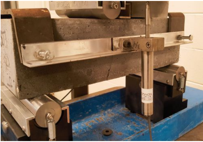
Figure 3. Verification of tensile properties of ultra-high-performance concrete through flexural testing. Photo and Figure: Wiss, Janney, Elstner Associates Inc.
