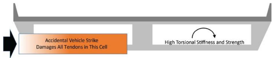
Figure 1. If one cell of a two-cell, three-span continuous post-tensioned concrete box girder is extensively damaged, the bridge would benefit from the high torsional strength and stiffness of the undamaged cell and continuity in the longitudinal direction. Figure: Dr. Oguzhan Bayrak.
