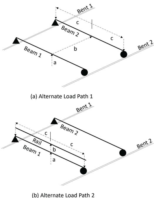
Figure 4. As a result of redundancies, two alternative load paths are available after a fascia girder, represented in the figure as beam 1, is heavily damaged near midspan. Figure: Dr. Oguzhan Bayrak.
