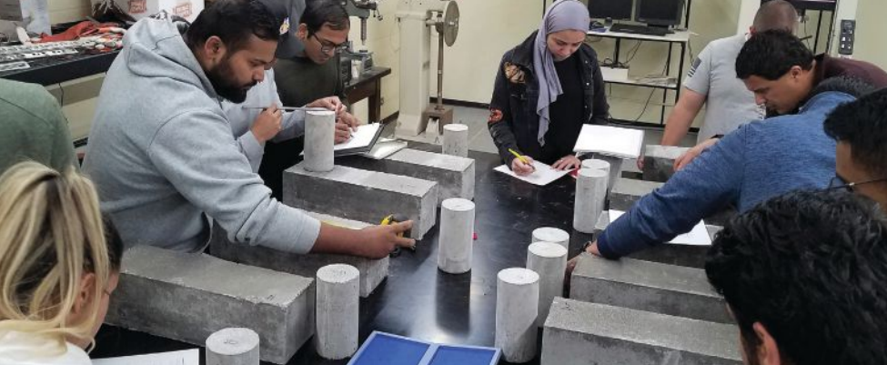
Students prepare concrete specimens for testing in the Idaho State University engineering materials laboratory.
