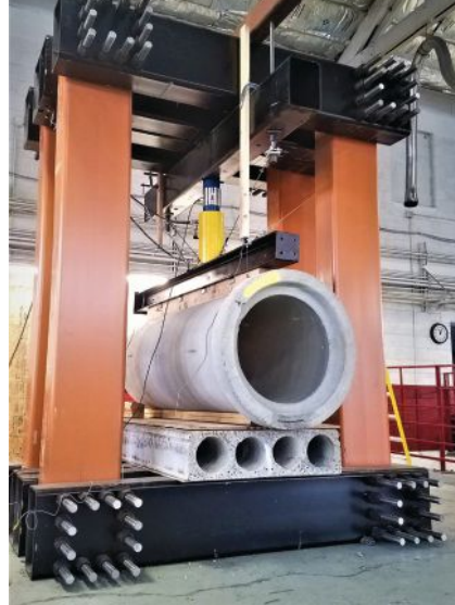
Full-scale testing of a precast concrete pipe.
