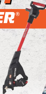
RB401T-E TIES #3 x #3, UP TO #6 x #6 With 19Ga. Wire
