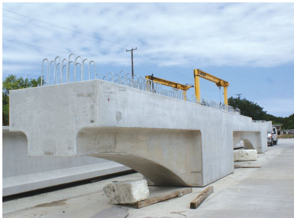
Figure 2. Variable-depth T-shaped precast, prestressed concrete hammerhead pier cap. Photo: Bexar Concrete Works.
