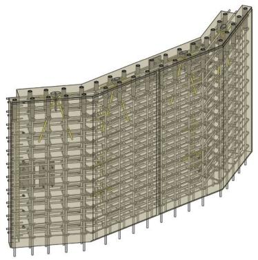
Elevation of a single, fully populated precast concrete panel of the tower (partial elevation view shown in the left figure). During erection, BIM is used to ensure that reinforcing bars extending from the bottom of the panel slide precisely into the grout sleeves in the panel below (not shown).
