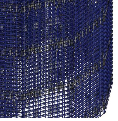
Partial elevation of a complex, densely reinforced precast concrete tower. With reinforcement, embedded handling hardware, and connections, the detailing of total-precast concrete structures can be challenging using conventional means. However, BIM was used from start to finish on this project to deliver it virtually error free.
