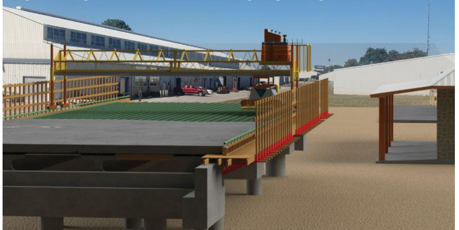
Figure 1. Rendering of the full-scale bridge deck construction mock-up to be used in the Concrete Bridge Engineering Institute’s Bridge Deck Construction Inspection Program. All Figures and Photos: Concrete Bridge Engineering Institute.
