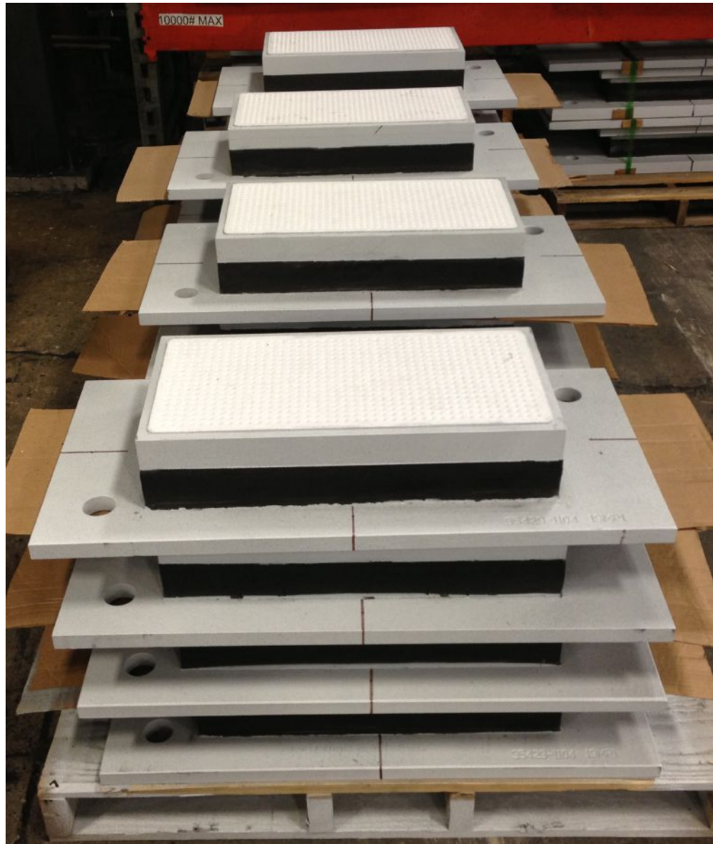
A low-friction polytetrafluoroethylene (PTFE) dimpled sheet, which is used as a sliding top surface on laminated elastomeric bearings. Dimples on PTFE surfaces function as reservoirs that receive lubricant before assembly.
