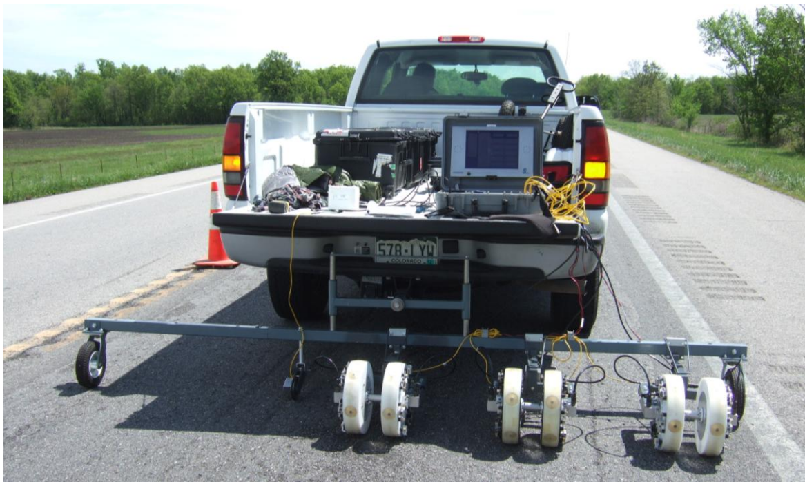
Figure 11 – Bridge Deck Scanner on Kansas Asphalt Pavement site with 3 pairs of wheels spaced 0.5 ft (0.15 mm) apart for combined Impact Echo and Spectral Analysis of Surface Waves scanning.
