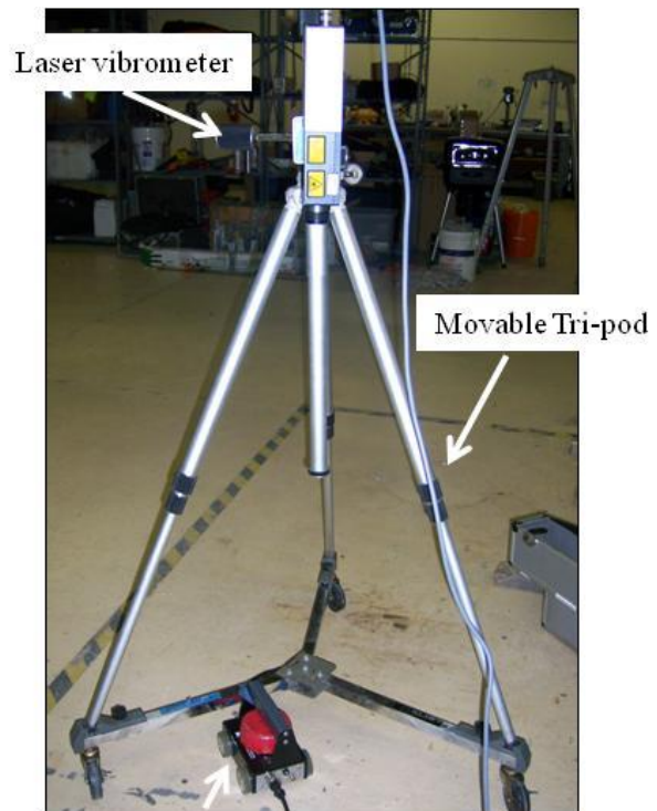
An automatic solenoid impactor (within the Impact Echo Scanner device) attached to the frame of the tri-pod
