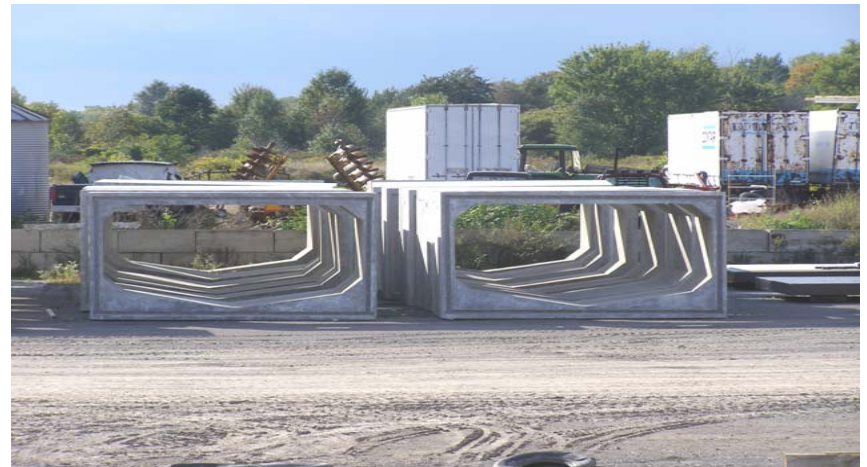
Culverts Fabricated at Kistner
