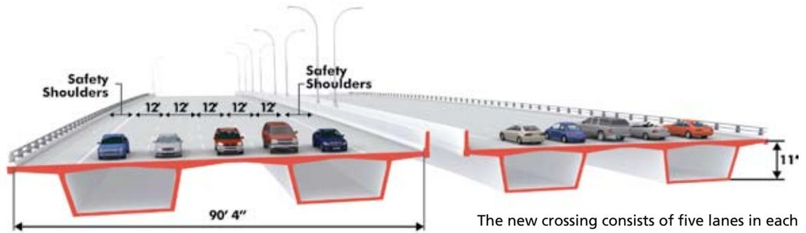
The new crossing consists of five lanes in each direction with standard width shoulders, and can accommodate a future light-rail transit system. Rendering: © FIGG.
