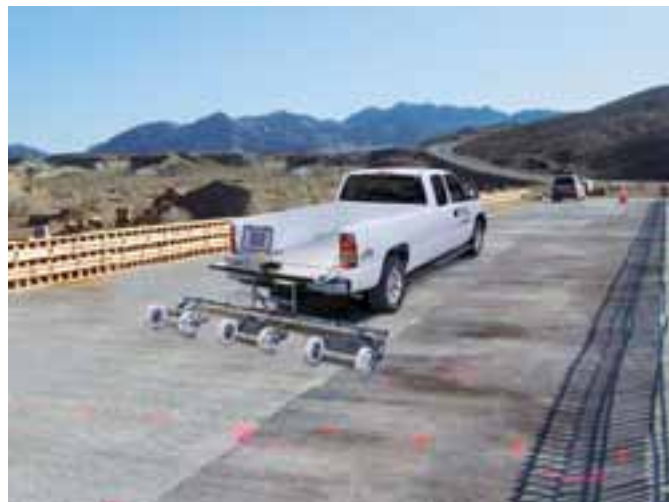
Bridge deck scanner conducting impact echo tests. Photo: Olson Engineering Inc.
