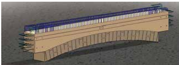
3-D representation of a typical column roof panel.
