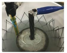
Grouted post-tensioning strand sample undergoing potentiostatic testing.
