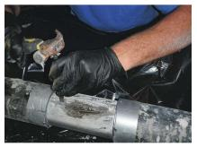
Removal of grout reveals impregnation material present on steel surface and penetration into surrounding grout.
