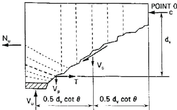
Figure 1. Anchorage of a longitudinal tie. AASHTO LRFD specifications C5.7.3.5-1.<sup>1</sup>
