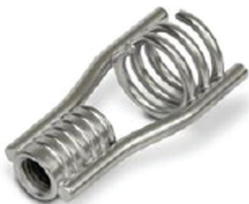
Figure 5. Proprietary concrete ferrule inserts are available from several manufacturers. Consult the specific manufacturer for capacities and installation requirements. For the Tenth Avenue Bridge project, the insert was threaded for 1¼-in.-diameter NC threads and had four struts instead of the two shown in this representative photo. Photo: Dayton Superior.
