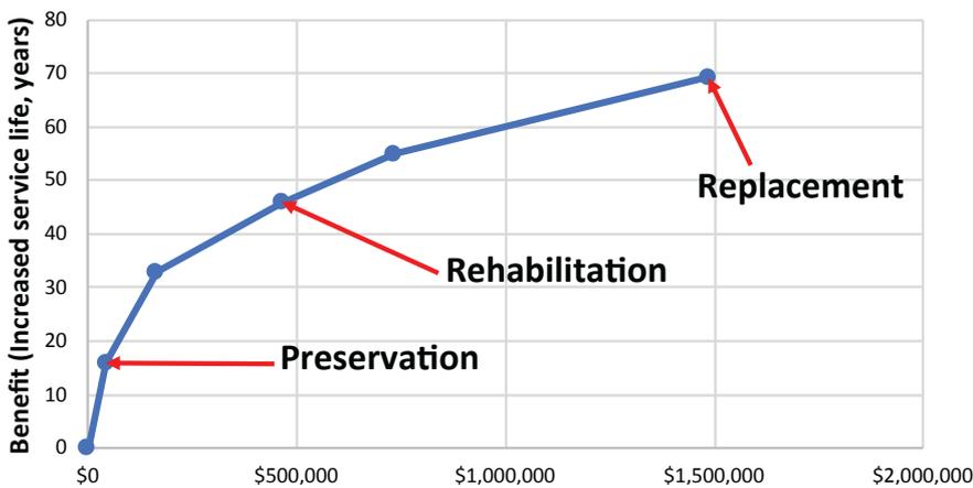
Figure 3. A benefit-cost comparison shows that well-chosen preservation actions can yield significant benefit at relatively low cost compared with rehabilitation or replacement projects. In this example, the benefit is measured in years of increased service life. Figure: Dave Juntunen.
