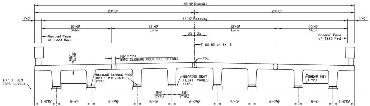
The bridge typical section shows the four NEXT 36 D beams, ultra-high-performance concrete closure joints, and the standard bridge width of 46 ft, which was used for all five bridges. The goal was to make the bridges as similar to each other as possible to optimize efficiency.
