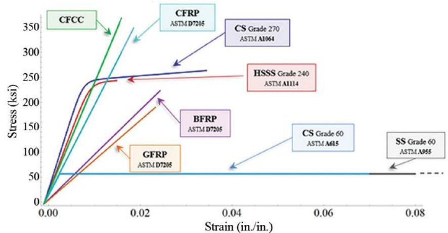
Figure 1. Comparison of the stress-strain relationships of several types of reinforcing bars and prestressing strands. Note: BFRP = basalt-fiber-reinforced polymer; CFCC = carbon-fiber composite cable; CFRP = carbon-fiber-reinforced polymer; CS = carbon steel; GFRP = glass-fiber-reinforced polymer; HSSS = high-strength stainless steel; SS = stainless steel. Figure: University of Houston.
