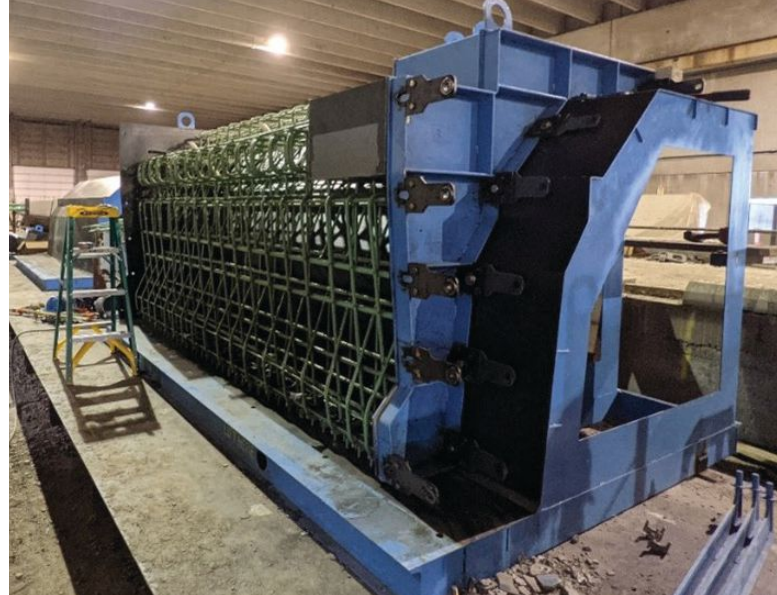
The fabrication form with near-side form removed shows epoxy-coated steel reinforcement in place for the casting of the moment slab. Self-consolidating concrete was used for all precast concrete components.
