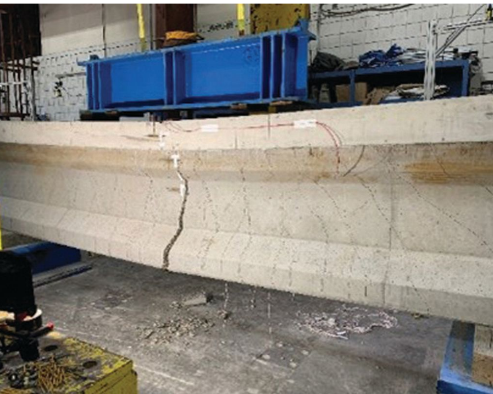
Figure 2. In a research study conducted for Florida Department of Transportation, 42-ft-long AASHTO Type II girders, all with 8-in.-thick, 24-in.-wide composite deck slabs and prestressed with stainless steel strands, were tested in flexure. 1 This photo shows a girder with nine strands immediately after failure by strand rupture. Girders with seven and eleven strands failed in the same manner.
