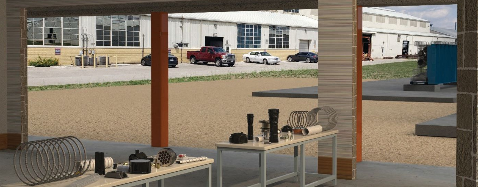
Figure 4. Course participants will be required to identify conforming and nonconforming components of post-tensioning systems as part of the post-tensioning system inspector module.
