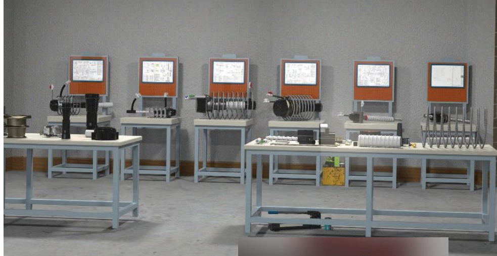
Figure 3 (above and on the right). Course participants in the Post-Tensioning Laboratory modules will be able to work with different types, brands, and sizes of post-tensioning systems, including both strand and post-tensioning bar systems.
